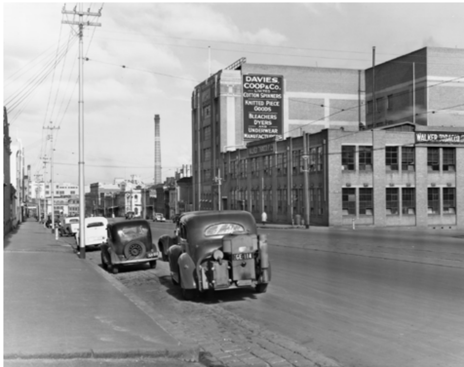
▲ A car with a charcoal burner attached on the back, taken in Swanston St, Carlton, opposite Lincoln Square, sometime in the 1940s. The tall chimney in the background is the one that is now inside the Melbourne Central shopping centre. Photo: State Library of Victoria.
